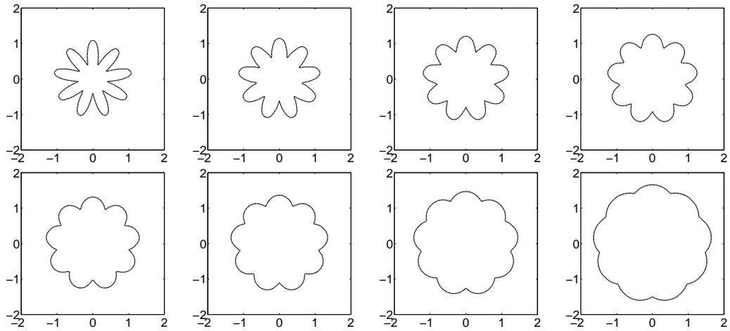
FIGURE 4.1. Evolution of a nine leaved rose-shaped interface as it moves normal to itself in the outward direction. The iteration number is written at each figures.
