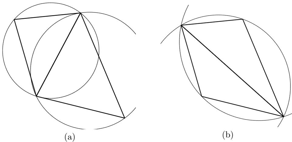
FIGURE 5.2. Delaunay Triangulation: (a) Correct and (b) Wrong
