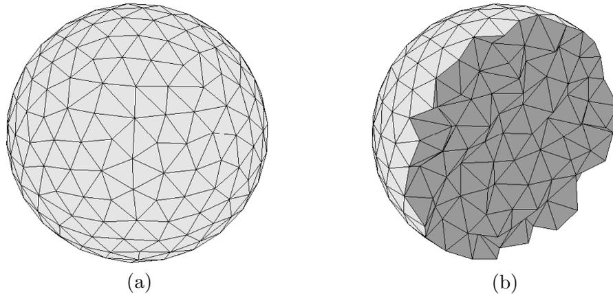
FIGURE 5.7. Unit Sphere mesh
