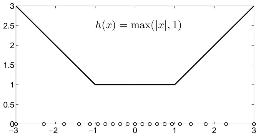
FIGURE 5.3. The relation between the mesh size function  $h(x)$  and generating mesh point length
