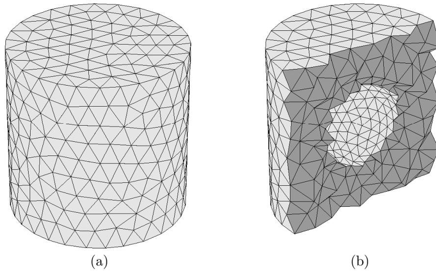
FIGURE 5.10. Cylinder with Spherical Hole
