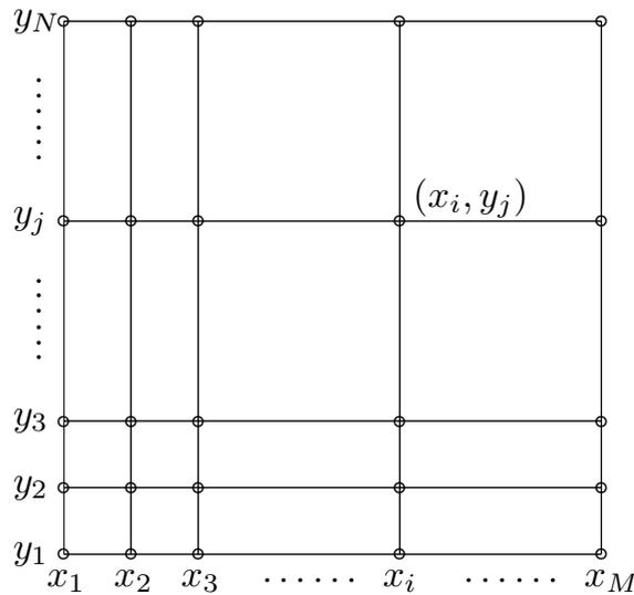
FIGURE 2.8. Two-dimensional cell corner mesh grid.
